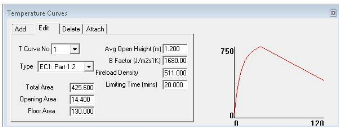
Figure 3.27. Parametric fire curve (EN1991-1-2) applied to the structure
