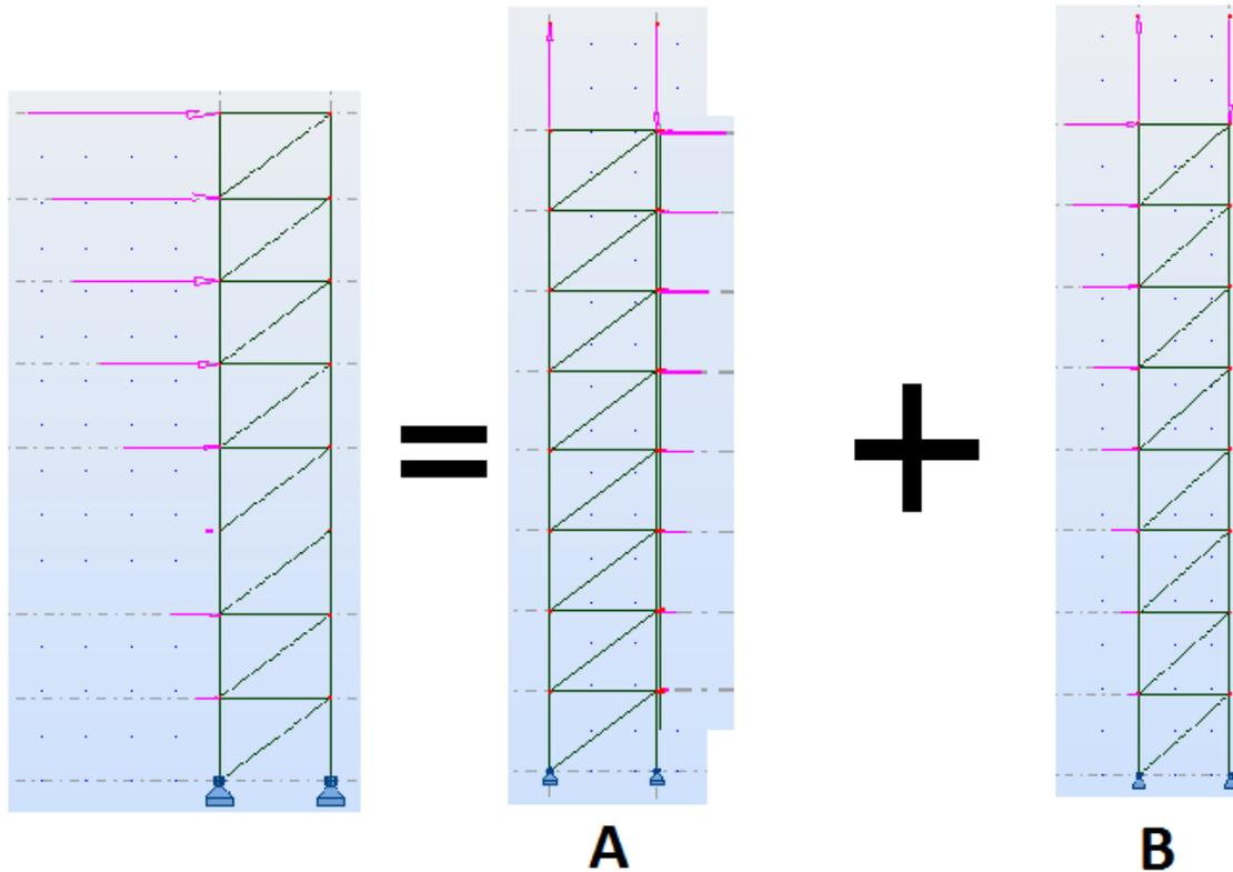
**Figure 32: Frame action superposition**
