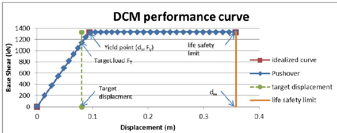
Figure 22: Pushover curve performance parameters
