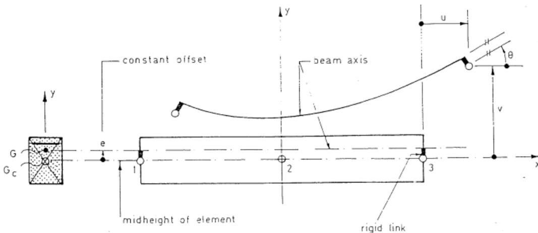
Figure 1 - BERNOULLI beam offset element
