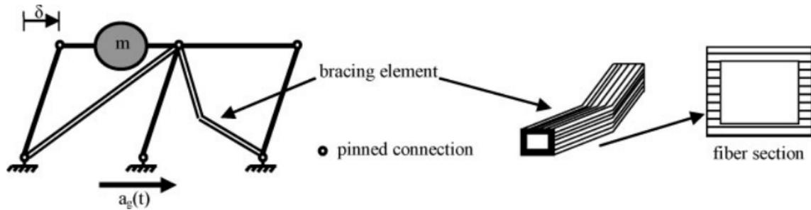
Figure 2: Model of an SDOF CB subjected to ground motion
