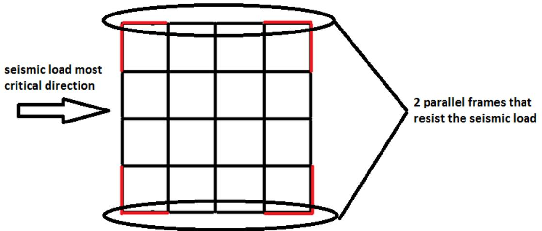
Figure 8: Assumed direction of seismic action on frames
