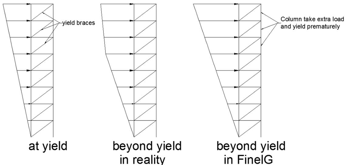
**Figure 37: Load distribution beyond brace yielding in reality and in FinelG model**
