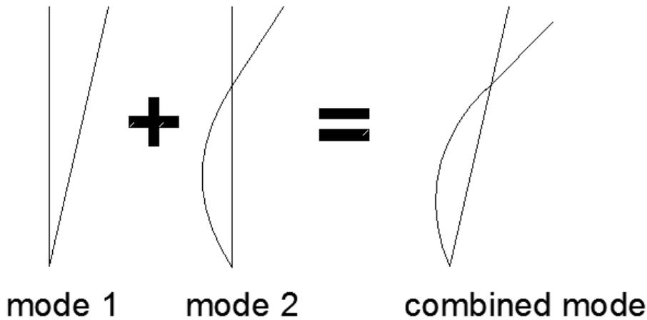
**Figure 43: Illustration on how mode 2 contribution can increase the top displacement**
