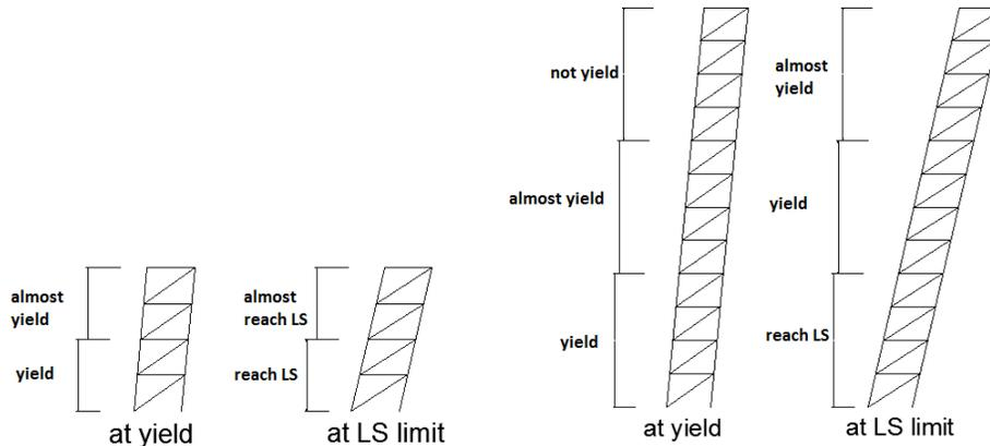
**Figure 35: Illustration of brace yielding pattern of 4 and 12 story building.**
