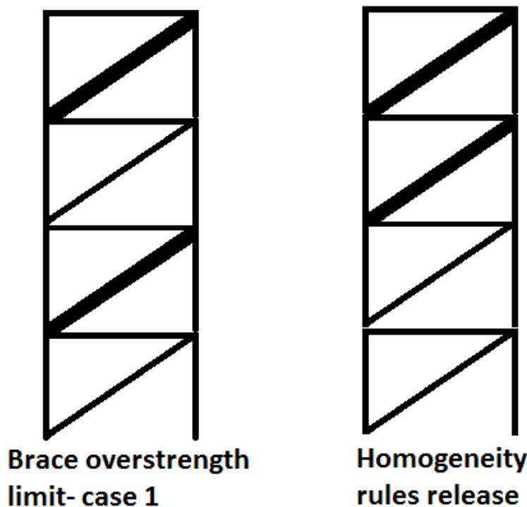
Figure 39: Comparison between 2 case studies, both has the weakest brace at the bottom floor
