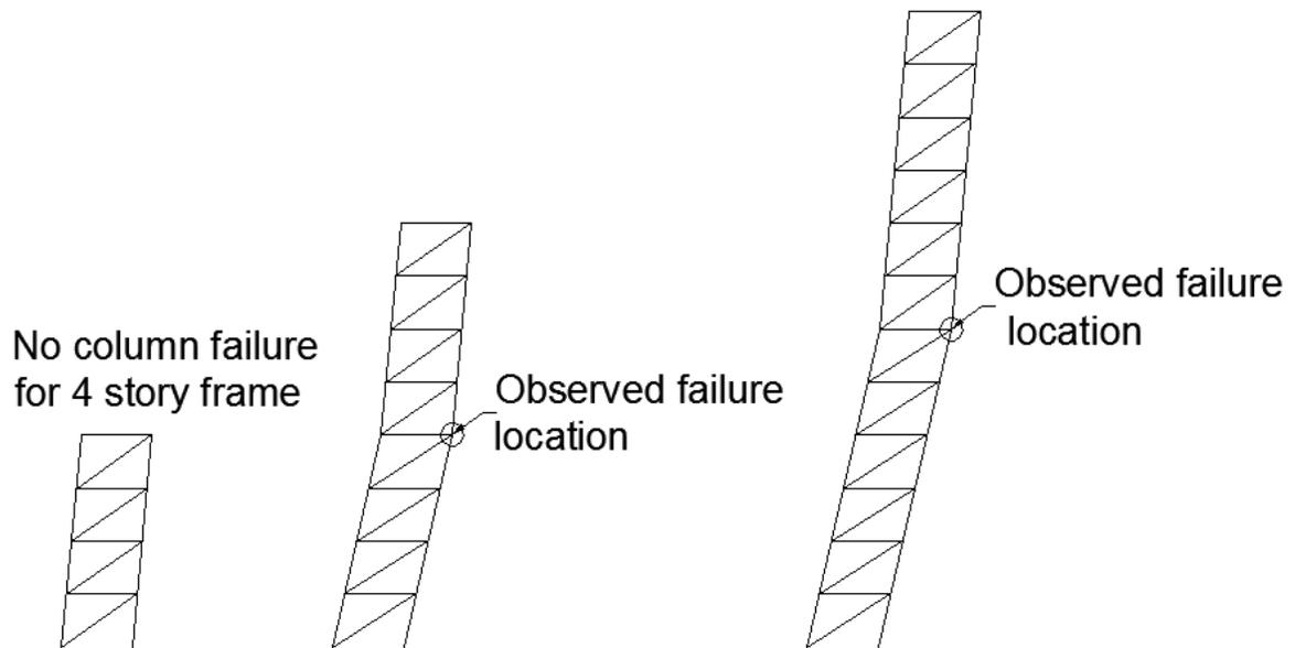
**Figure 40: Frame behavior with column failure when W<sub>max</sub>/W<sub>min</sub>=1.7**
