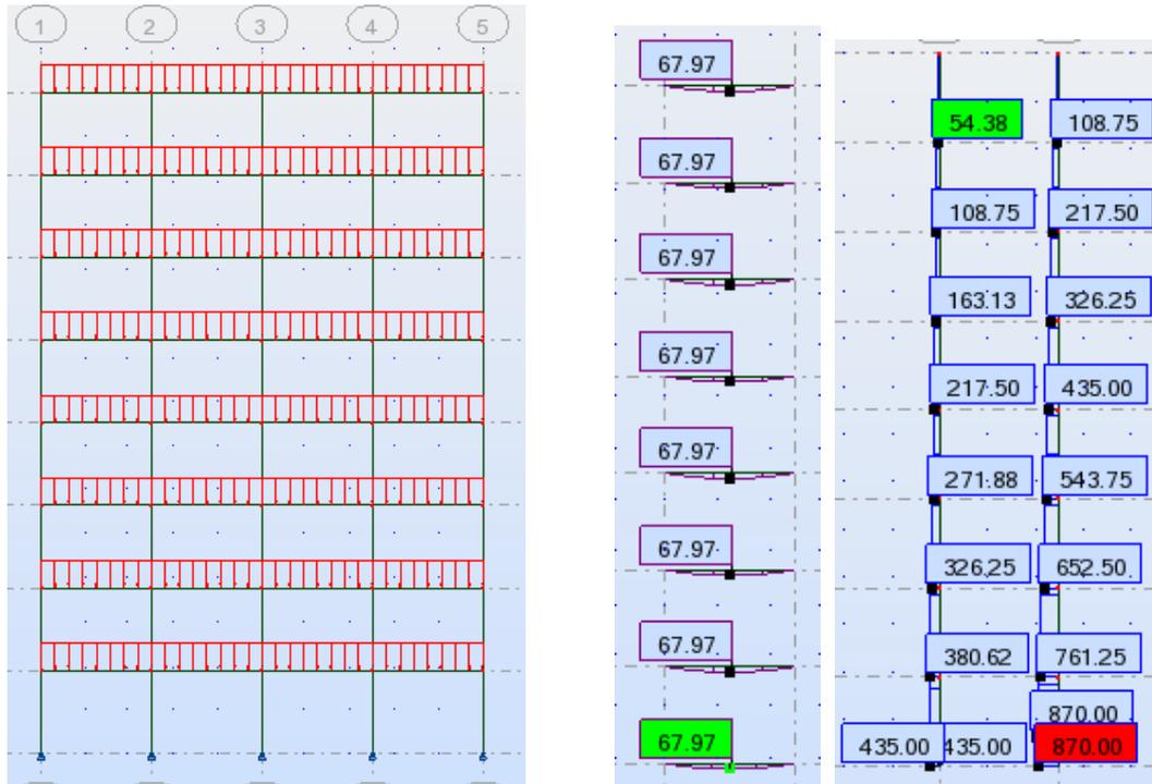
Figure 11: Frame internal load under gravity load
