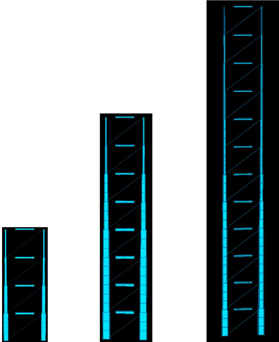
**Figure 17: FinelG model for different numbers of story (4/8/12)**
