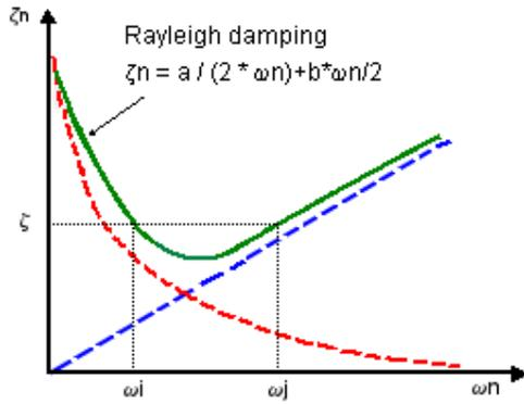
**Figure 24: Rayleigh damping Matrix**
