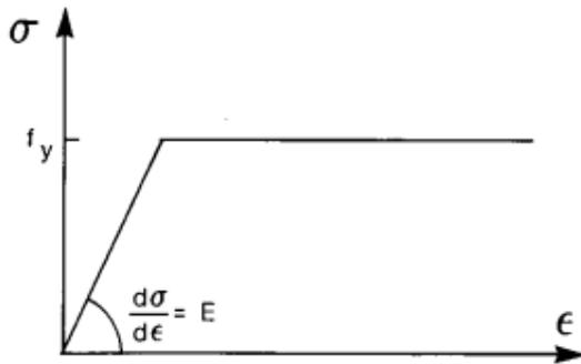
Figure 6: Bi-linear stress-strain relationship
