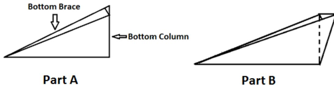
In Part A, assuming the column utilization factor is almost 1, the induced stress in the brace can be calculated as following (column height is 3.75m, brace length is 6.25m, the angle between them is 53o)
