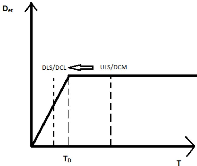
**Figure 34: Variation of target displacement against structural stiffness**
