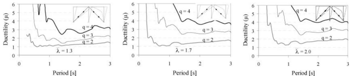
Figure 4: Ductility demands on braced frames in soft soils
