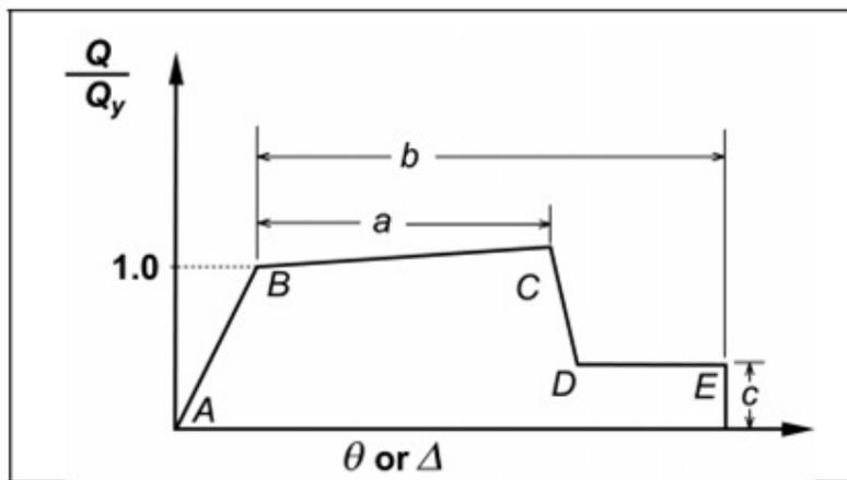
Figure 20: generalized force-deformation relation for steel elements or components
