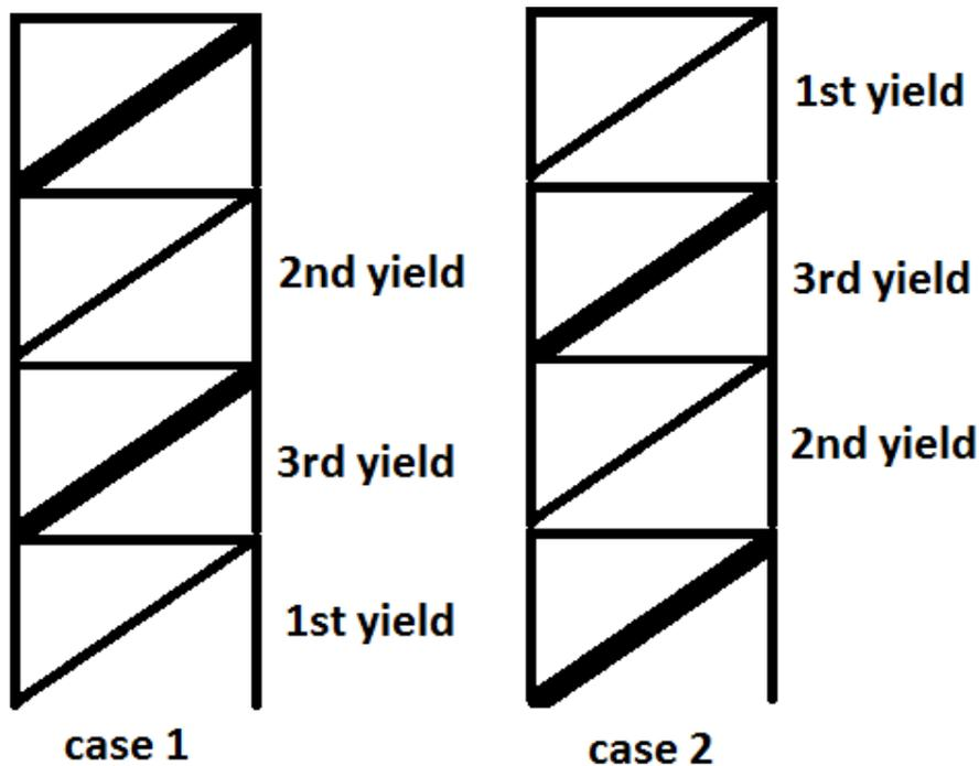
Figure 36: Two brace-overstrength configurations and yielding sequence as noted by order
