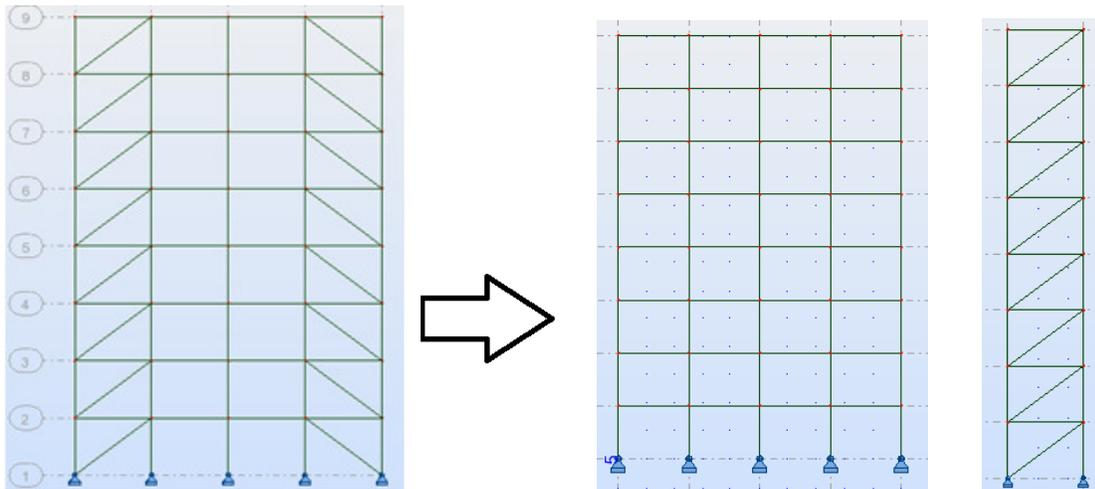
**Figure 10: Simplified Structural Layout for gravity load (middle) and lateral load (right)**
