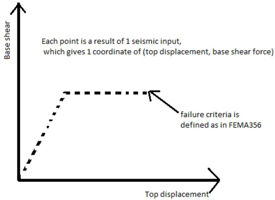
Figure 38: Predicted result of dynamic analysis with incremental seismic input
