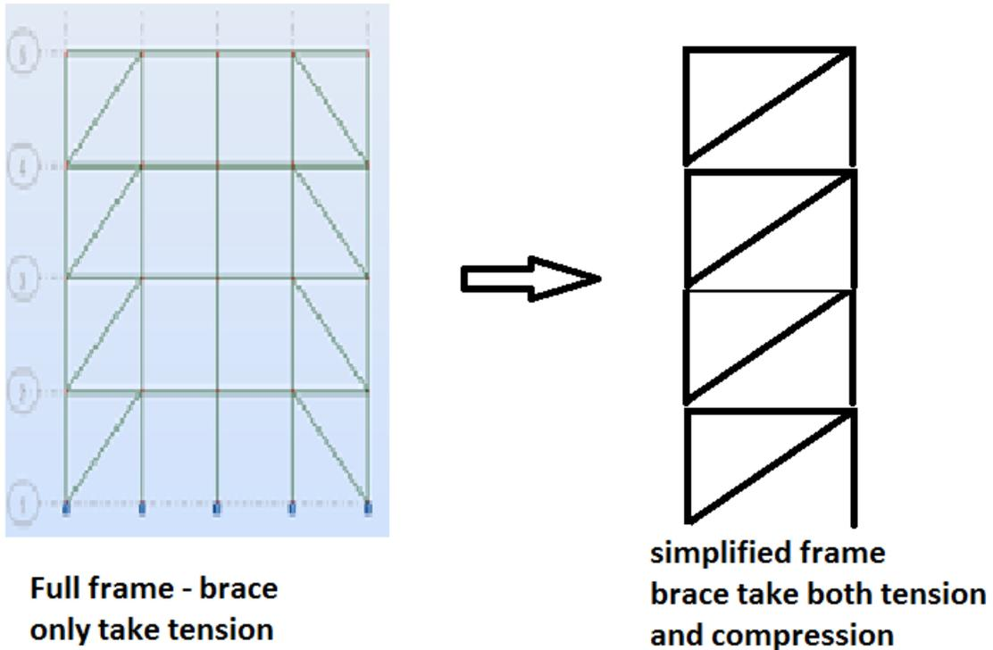
**Figure 25: Transformation from full frame to to simplified frame for dynamic analysis**
