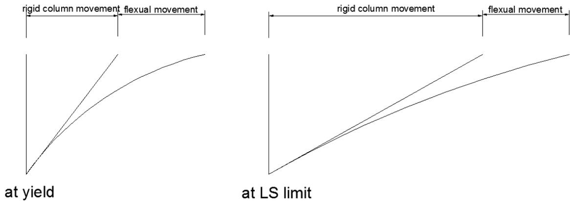
**Figure 41: Total displacement contribution from rigid and flexural movement of the column**
