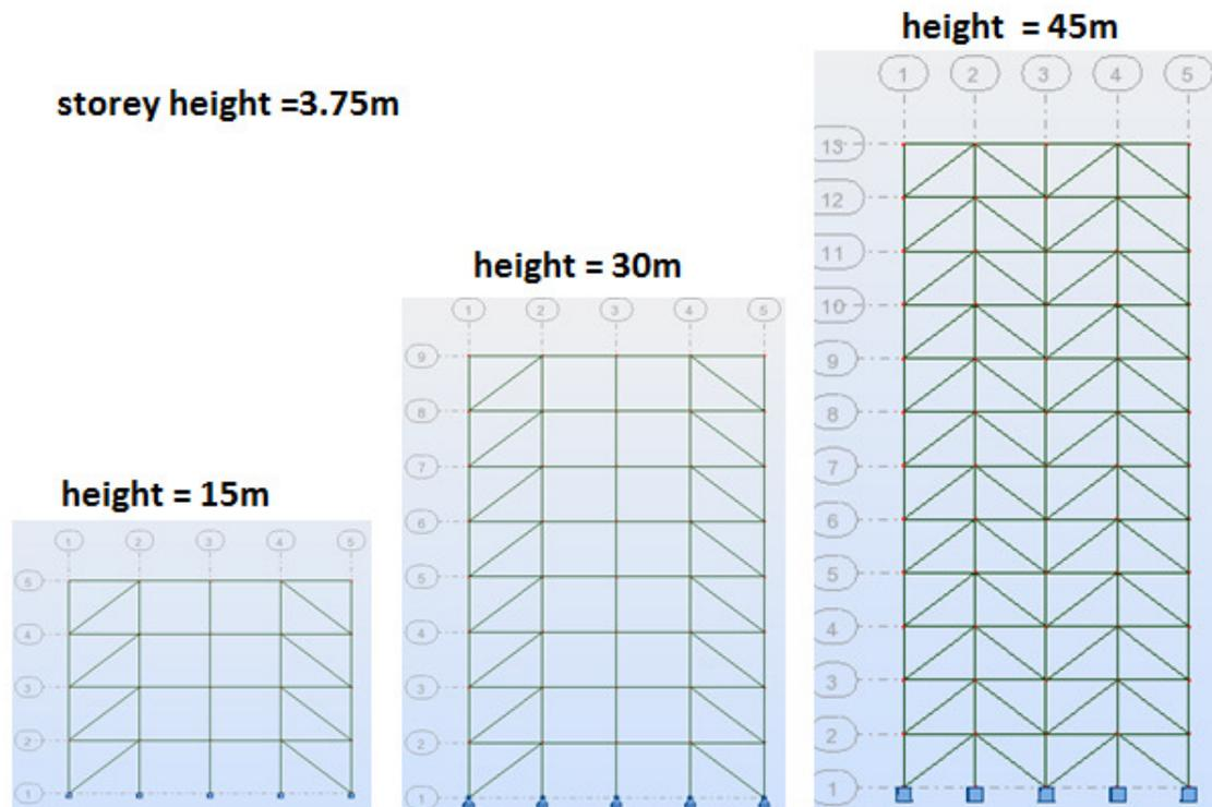
**Figure 7: Structural layout for 4/8/12 story structure**
