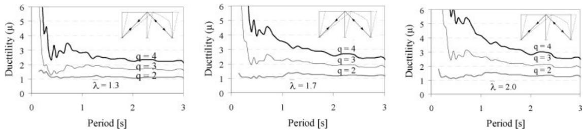
Figure 3: Ductility demands on braced frames in stiff to moderately stiff soils
