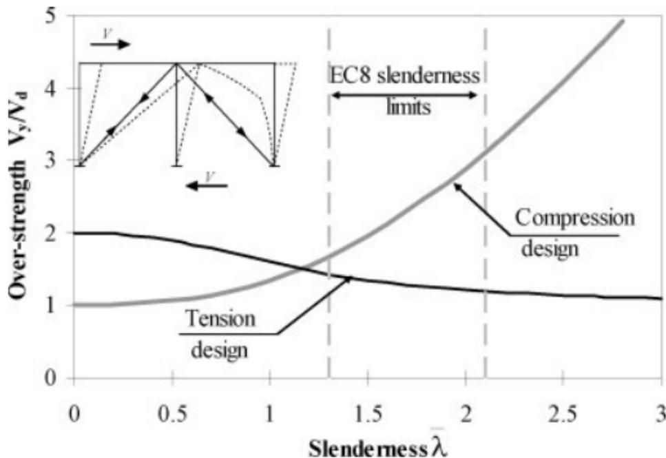
**Figure 1: Variation of frame overstrength with brace slenderness (Elghazouli, 2011)**
