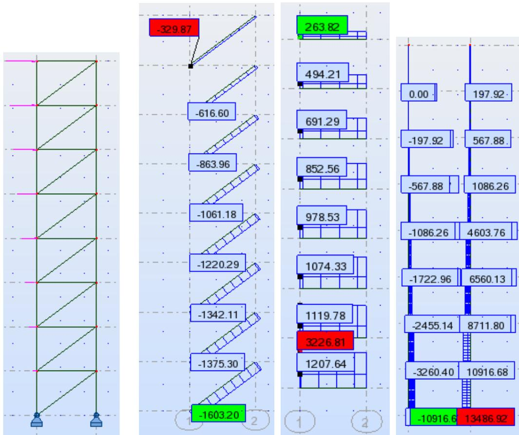
Figure 12: Frame internal load under the seismic action
