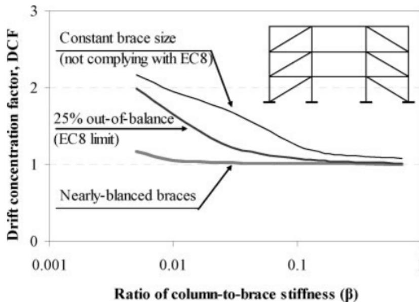
Figure 5: How column stiffness influences inelastic demand (Elghazouli, 2011)
