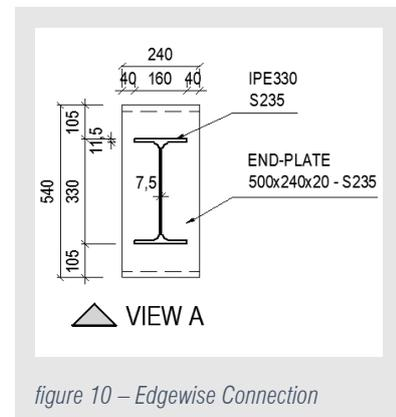
figure 10 – Edgewise Connection
