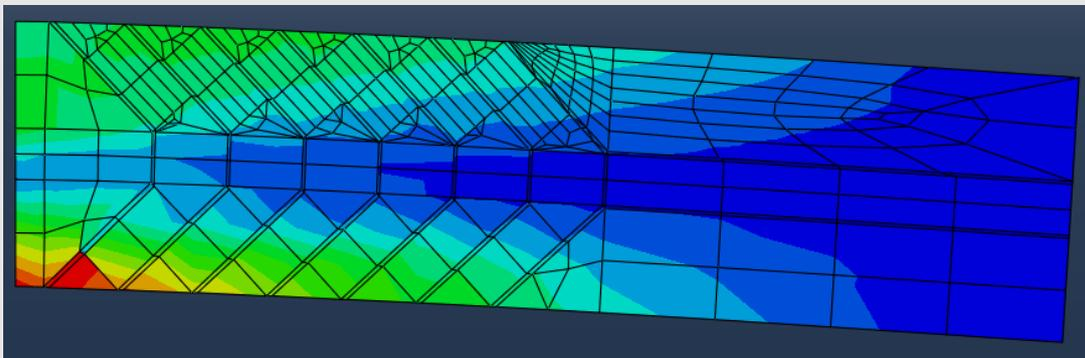
*figure 31 – Glulam beam model - Deformed shape amplified with a scale factor of 3*
