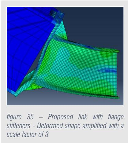
It can be evaluated that the **ductile mechanism** will be favored in relation to the other elements involved in the connection, avoiding specially the brittle collapse, proof that they have sufficient strength. The energy is being dissipated by the steel link confirming the theoretical prediction. The results open a way to an improvement of this technology focused on the seismic resistant performance of timber structures.
