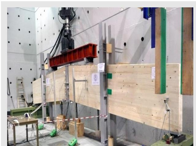
figure 26 - ENEL's Dome - 4-point bending test realized at University of Trento (Mazzolani's photography)
