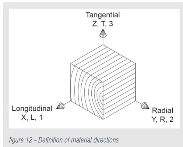
figure 12 - Definition of material directions
