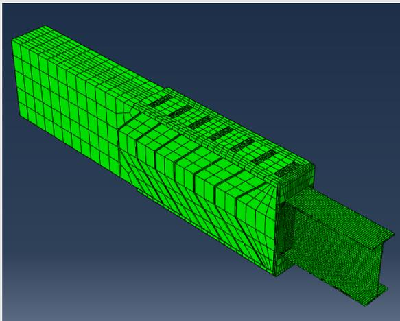
figure 29 – Steel link and proposed connection modelled with timber as isotropic
