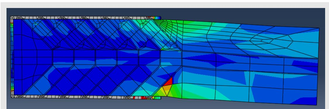
figure 30 – Connection model - Deformed shape amplified with a scale factor of 3
