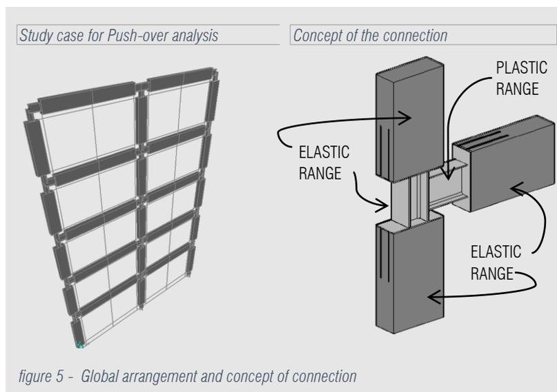
figure 5 - Global arrangement and concept of connection
