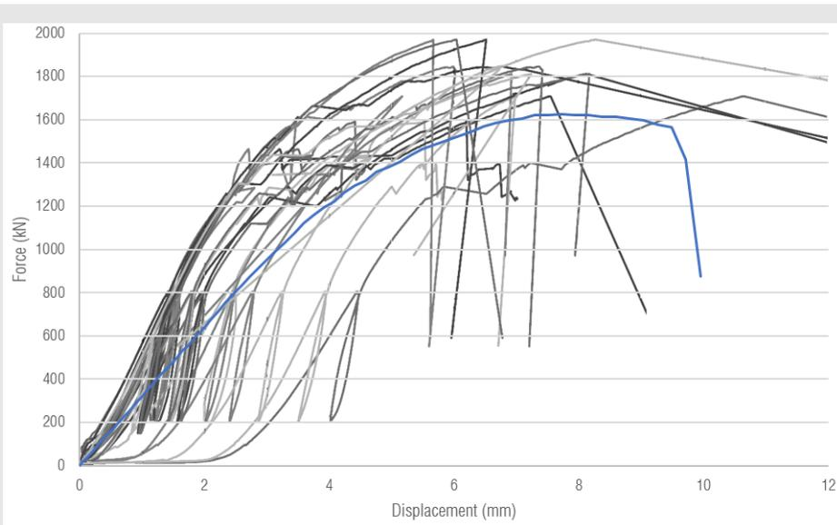
figure 25 – Tension test – Abaqus output compared with the range of results from the experimental tests
