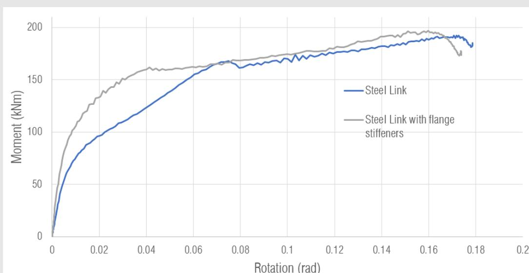
figure 34 – Moment-rotation curve of the proposed connection - Abaqus output
