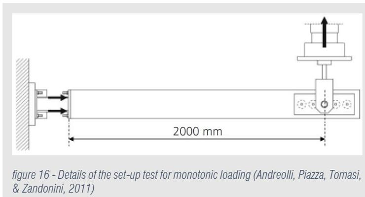
Fixed **boundary conditions** were imposed to the free end-plate. The free end of the timber beam starts from a steady-state condition and is subjected to a controlled displacement applied smoothly through the whole step time.
