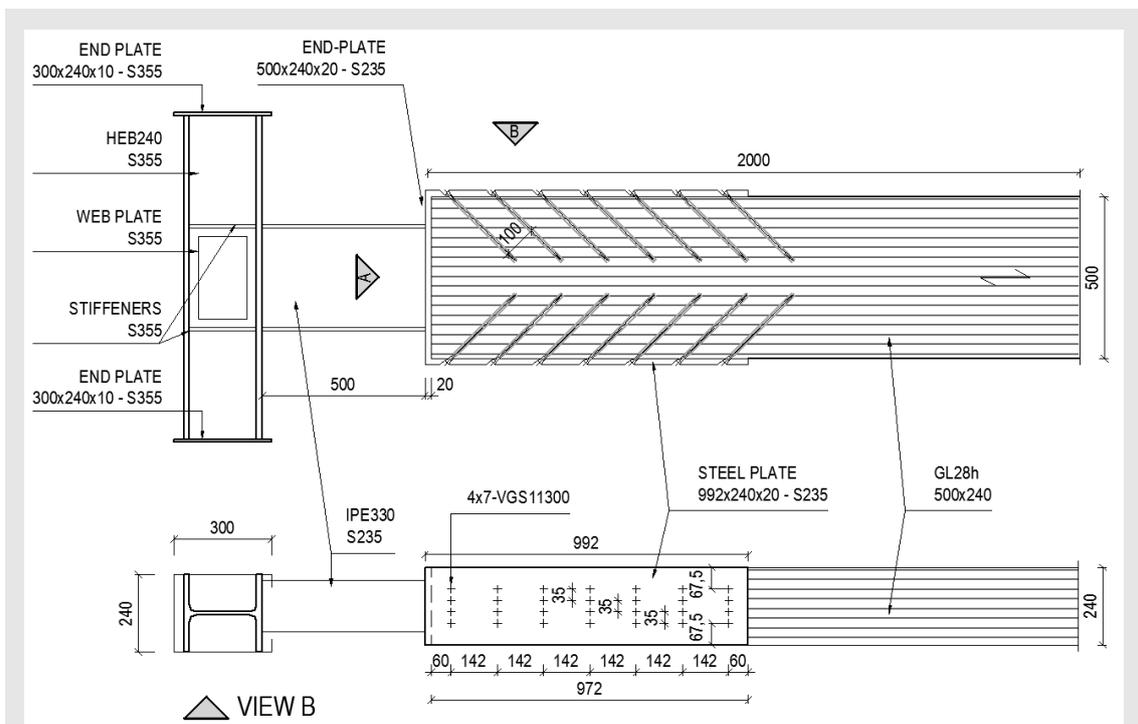
figure 11 – Edgewise Connection
