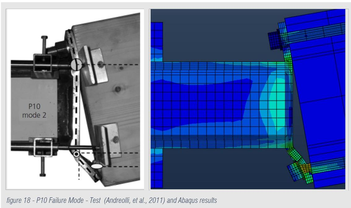
figure 18 - P10 Failure Mode - Test (Andreolli, et al., 2011) and Abaqus results
