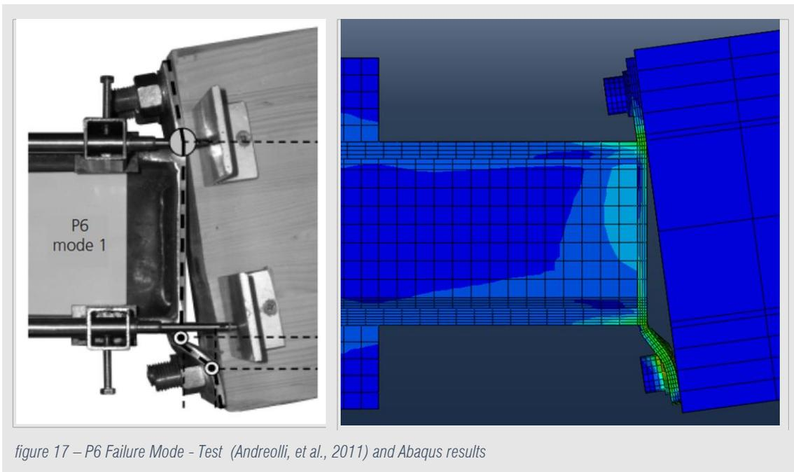
figure 17 – P6 Failure Mode - Test (Andreolli, et al., 2011) and Abaqus results
