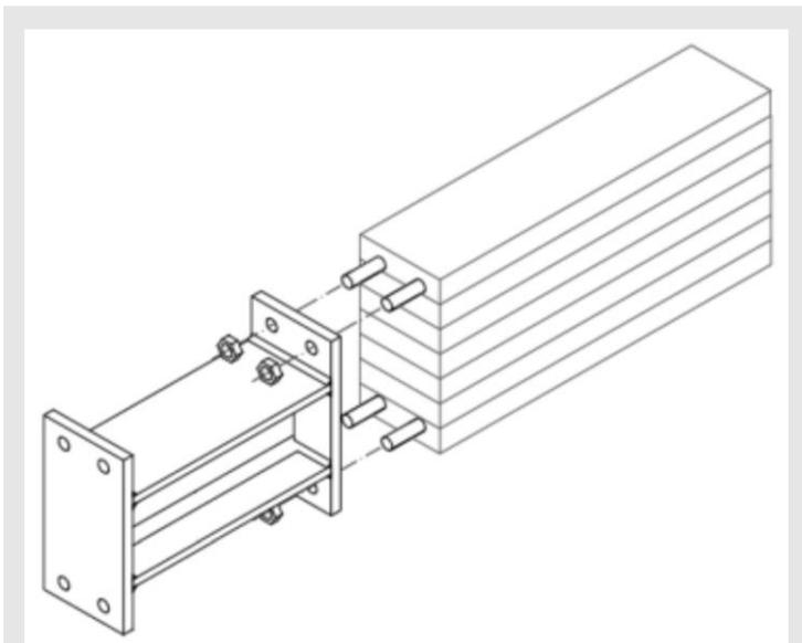
figure 7 - University of Trento's tested seismic link (Andreolli, Piazza, Tomasi, & Zandonini, 2011)
