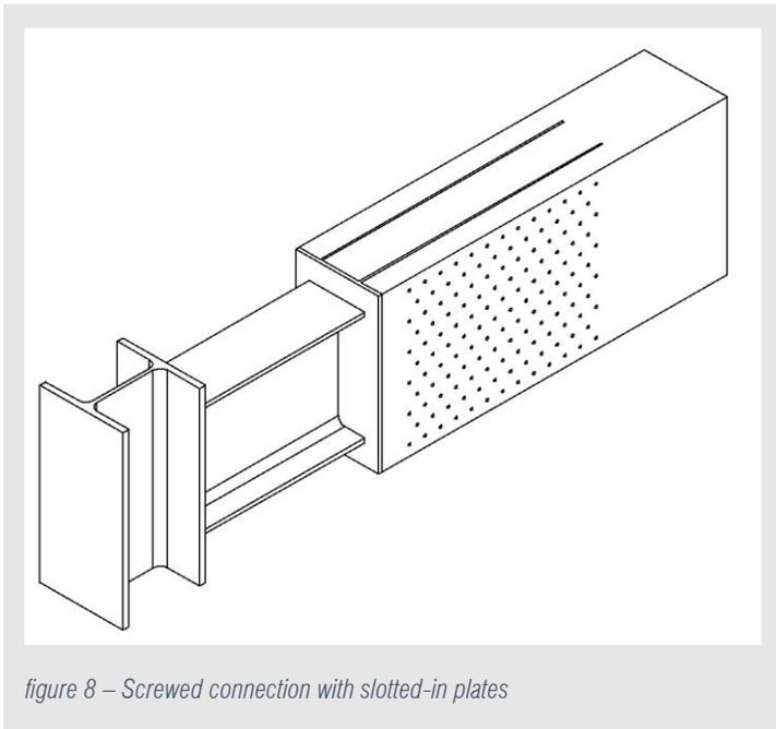
figure 8 – Screwed connection with slotted-in plates
