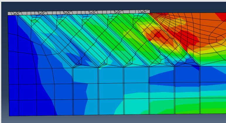
figure 24 – Tension test – Abaqus failure mode
