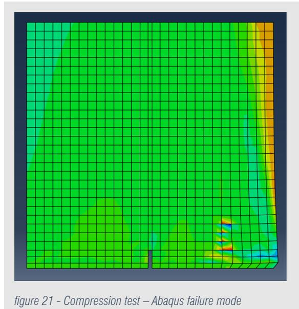
figure 21 - Compression test – Abaqus failure mode
