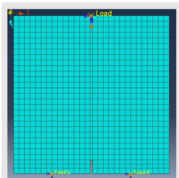
figure 20 - Compression test - Material orientation and boundary conditions
