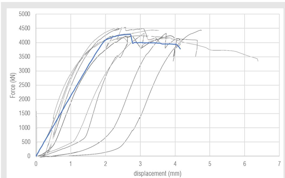
figure 22 - Compression test – Abaqus output compared with the range of results from the experimental tests
