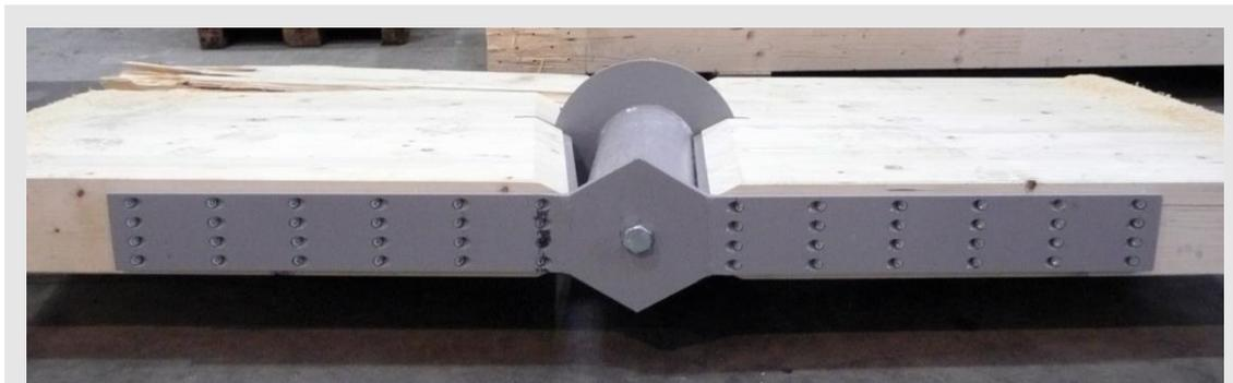
figure 9 – Edgewise connection of ENEL's Dome - University of Trento (Mazzolani's photography)
