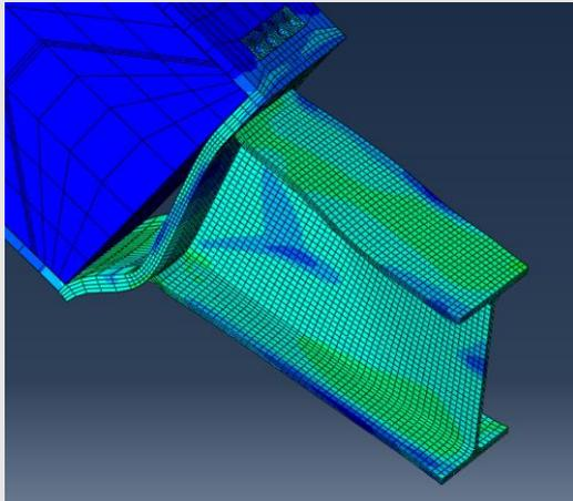
figure 33 – Proposed link – Deformed shape amplified with a scale factor of 3
