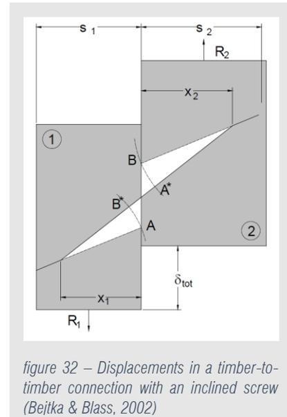
figure 32 – Displacements in a timber-to-timber connection with an inclined screw (Bejtka & Blass, 2002)
