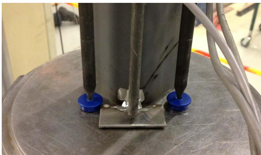
Figure 8.2.4: Additional plate welded to the specimen for installation of LVDT1. Magnets used for LVDT3 and 4.
