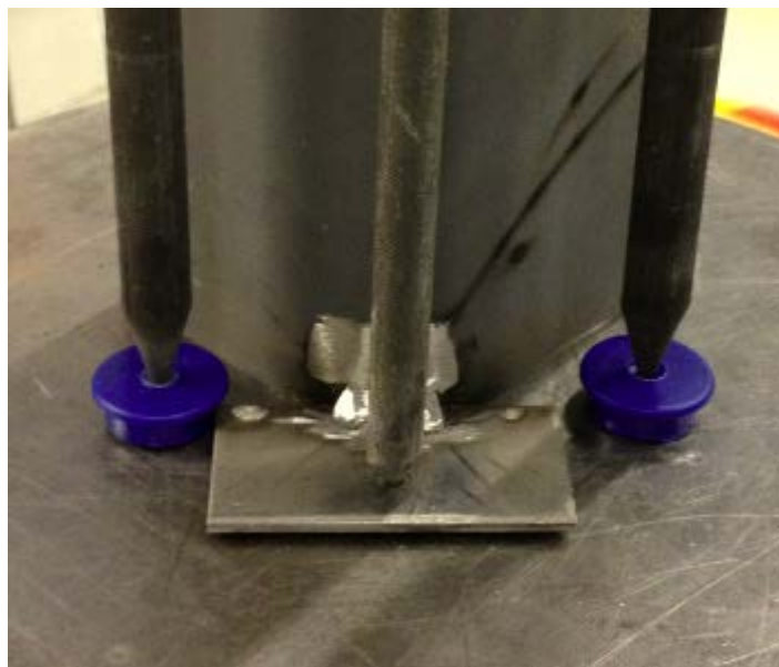
Figure 10.1.6: Final solution, LVDT 1 welded to the specimen
