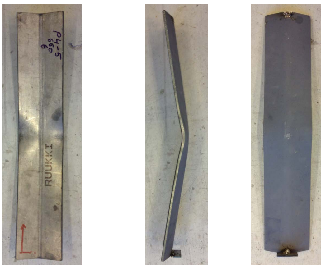
Figure 8.2.7: Deformation of specimen P4-5-6mm (typical failure for P4-6).
