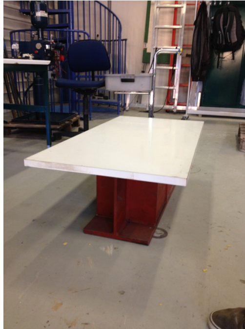
Figure 8.1.5: Stable base for positioning of specimens
