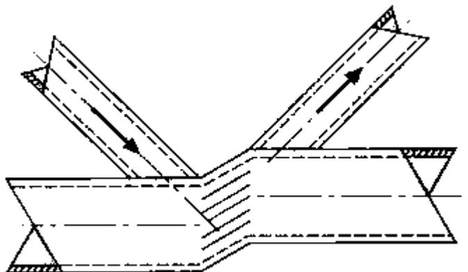
Overall shear failure of the chord
