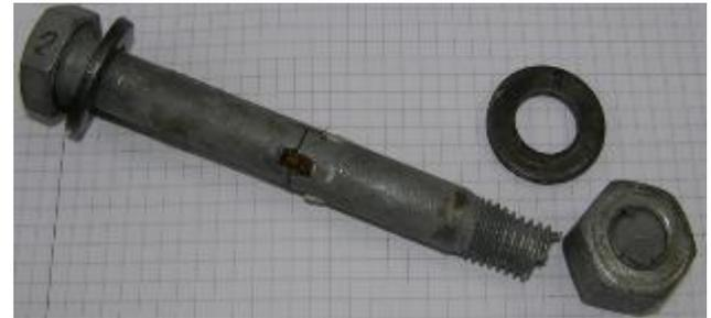
Rupture of bolt close to nut
