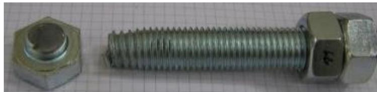
Rupture of bolt close to head
