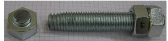
Rupture of bolt close to head
