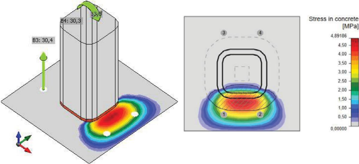
Fig. 8.4.3 CBFEM results for point 0, e.g. pure bending moment
