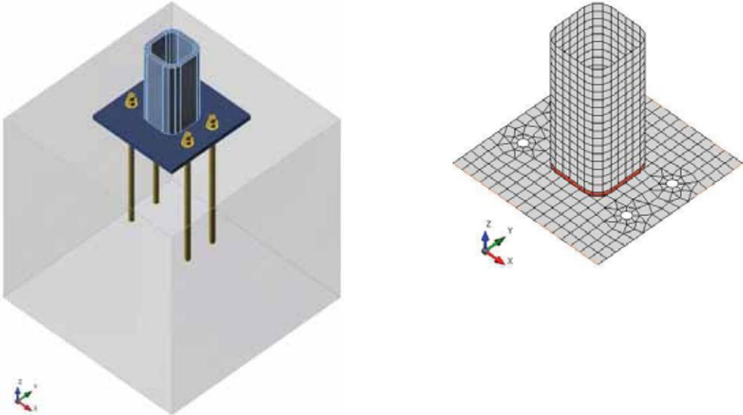
Fig.8.4.2 The column base for column SHS 150x16 and selected meshed of base plate
