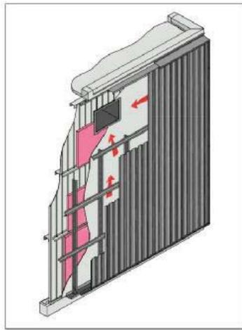
SolarWall® system mounted over metal wall
