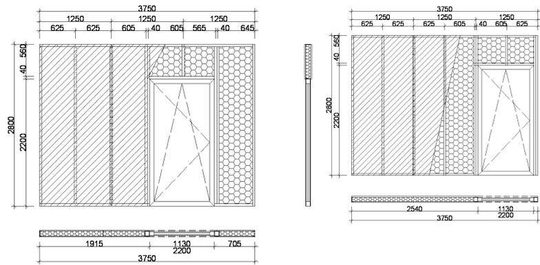
STRUCTURE OF BUILDING PANEL AND INSULATION THICKNESS 120 mm
