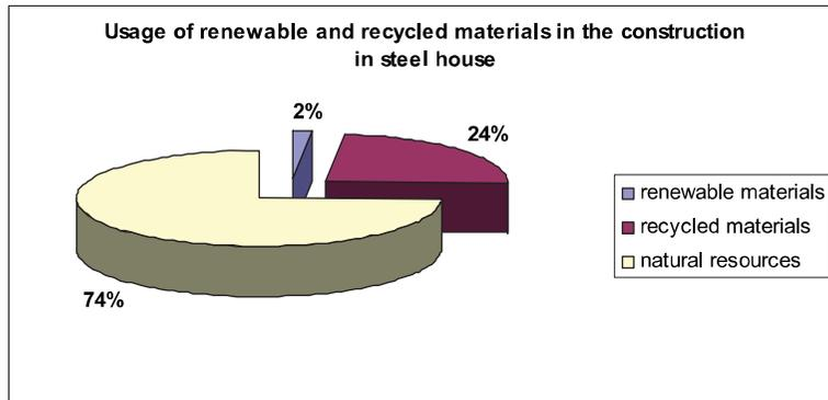
**Usage of renewable and recycled materials in the construction in steel house**
