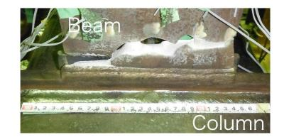
+4  $_{b}\theta_{p}(2)$  Crack Initiation at weld access hole +8  $_{b}\theta_{p}(1)$  Fracture at Beam flange
