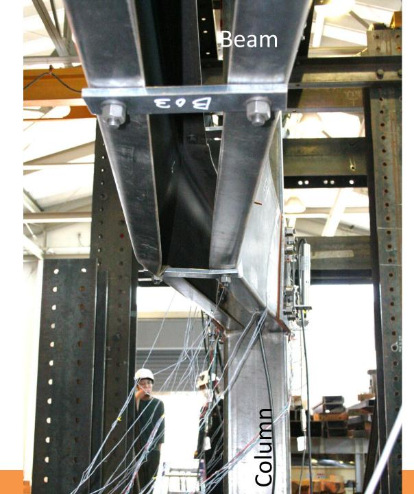
Failure mode observed in Special Bolted Moment Frame (SBMF)
