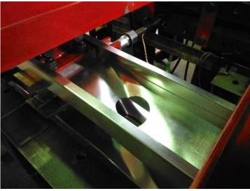
Deformed Shape -Burring OPENING-
