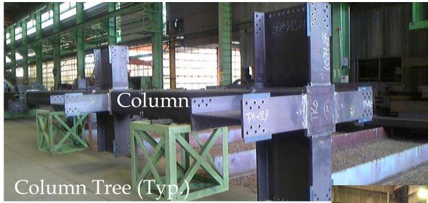
Shop Welded Detail ✓ Column Tree ✓ CJP ✓ UT inspection
