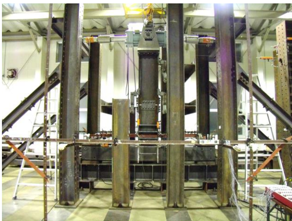
Fig. 1. Beam-to-column connection test setup
