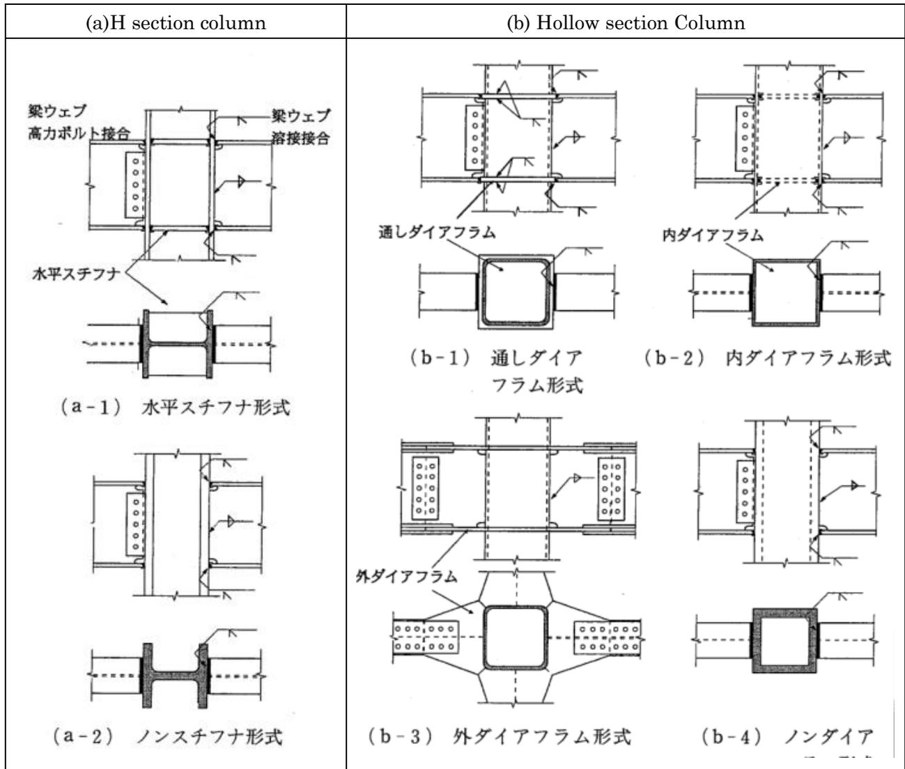
Figure C2.1 Typical rigid beam joint
