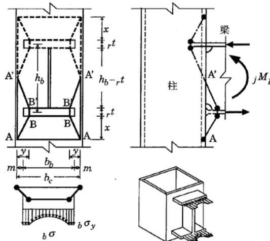
Figure C2.5 Failure mechanism at the column flange
