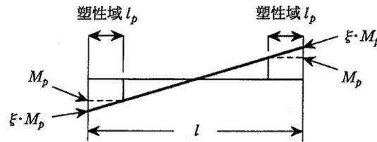
Figure C2.2 Plastification of the Beam ends during seismic event and hardening effects
