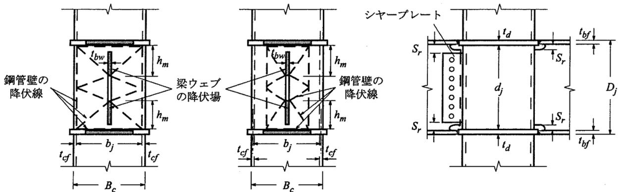
(a) Rectangular Hollow Section      (b) Circular Hollow Section      (c) Elevation of Connection
