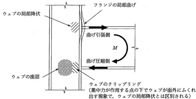
Figure C2.4 Local failure at the beam joint where continuity plates are not installed
