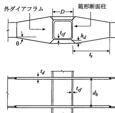
Figure 2.3 External Diaphragms for beam-to-column connection
