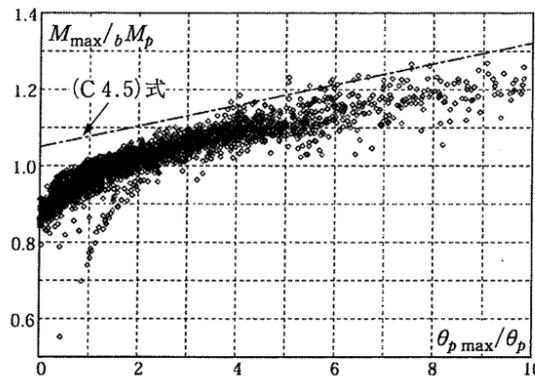
Figure C2.3 Hardening effect due to plastic deformation of the beams
