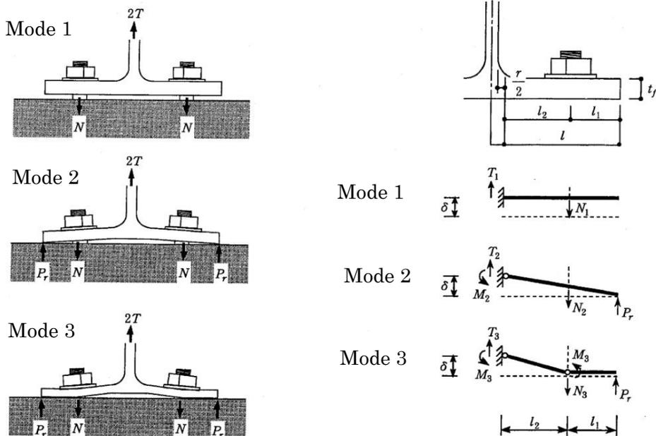
Figure C2.6 Local deformation and Failure modes at T-stub
