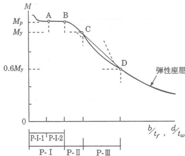
Figure C3.1 Classification of Cross Section
