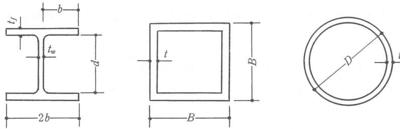
Figure 3.1 Geometrical symbols defined for cross-sections
