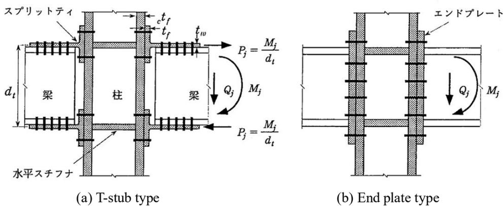
Figure 2.4 Beam joints by high-strength bolts
