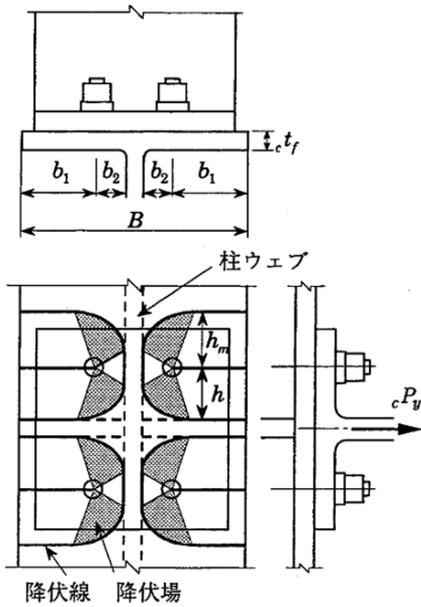
Figure 2.5 Failure mechanism at H-column flange
