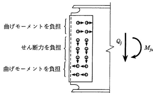
Figure 2.2 Force distribution in the beam web joint (high-strength bolted joint)
