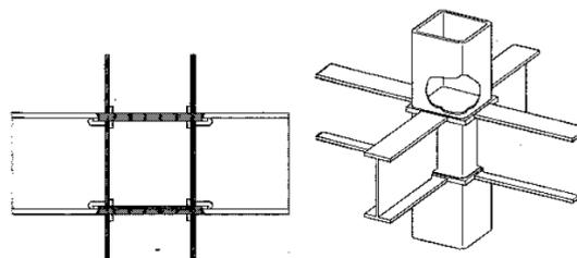
Figure 1.2.1 Typical Beam-to-Column Connection
