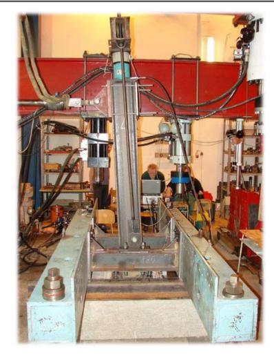
Set up in uniaxial bending
